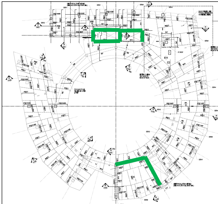
Figure 7: Shear wall locations
